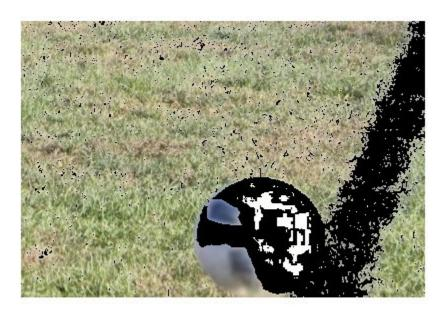
White pixels are partially removed from the border and ball segments. The green segment also incorrectly includes pixels from the ball. Therefore, the classification process requires another pixel attribute that can identify the difference between the grass field and the ball.
